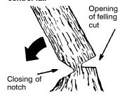
**NOTE:** Before felling cut is complete, use wedges to open the cut when necessary to control the direction of fall. To avoid kickback and chain damage, use wood or plastic wedges, but never steel or iron wedges.
